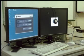
RadiCS can run tests for both AAPM and DIN acceptance standards, and the AAPM, DIN, JIS and IEC constancy standards.
