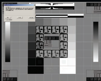
RadiCS performs easy confirmation of pattern, brightness, contrast and uniformity checks. Administrator workload is also reduced.
